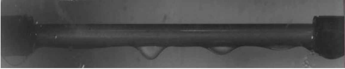
Figure 7.4: Image of filmwise condensation at saturation conditions, on a smooth copper tube (92 mm length) treated with hydrogen peroxide ( H_2O_2 ).
