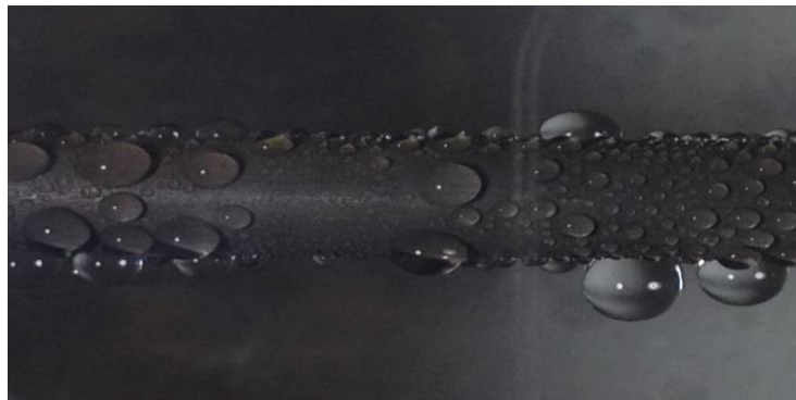
Figure 7.23: A photograph image of cuprite coating treated with H 2 O 2 / SAM , polished and then treated secondly with SAM for about 15 min. The color changed from red to more reddish and then to black after the H 2 O 2 treatment, which is similar to the color of the copper oxide surface.
