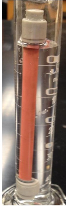
Figure 7.27: A photograph image of the yellow copper surface prepared by cleaning the cuprite coating ultrasonically in sulfuric acid, acetone, and ethanol, respectively.
