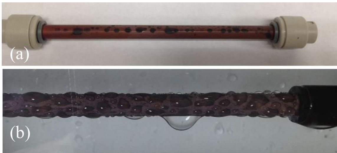
Figure 8.14: Photographic images of (a) the cuprite surface coated partially with irregular copper oxide coating and (b) the behavior of the dropwise condensation on the damaged surface when starting the condensation experiment with steam temperature and pressure higher than the saturation conditions.
